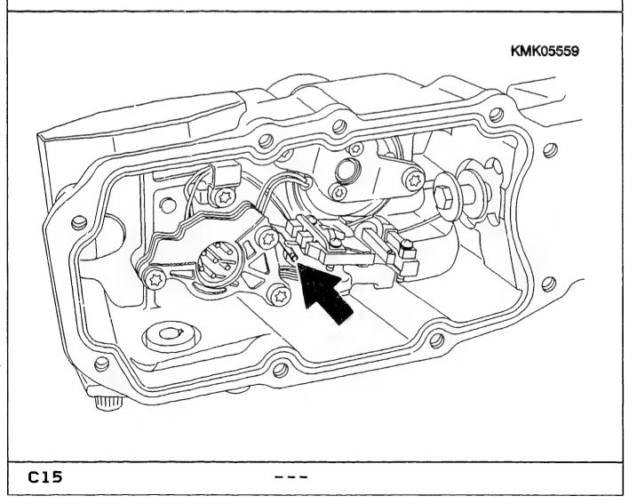
Replacing 7-pin terminal board:
